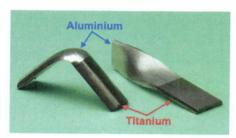
elevated temperature (about 50%-90% of the absolute melting point of the parent material) using an applied pressure for a time ranging from a few minutes to a few hours.
